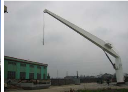
HOSE HANDING CRANE (DH)
